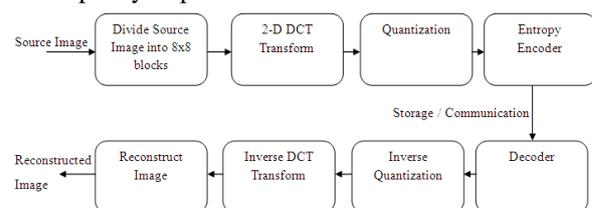
figure.3: Block Diagram For Compression/ Decompression Algorithm
